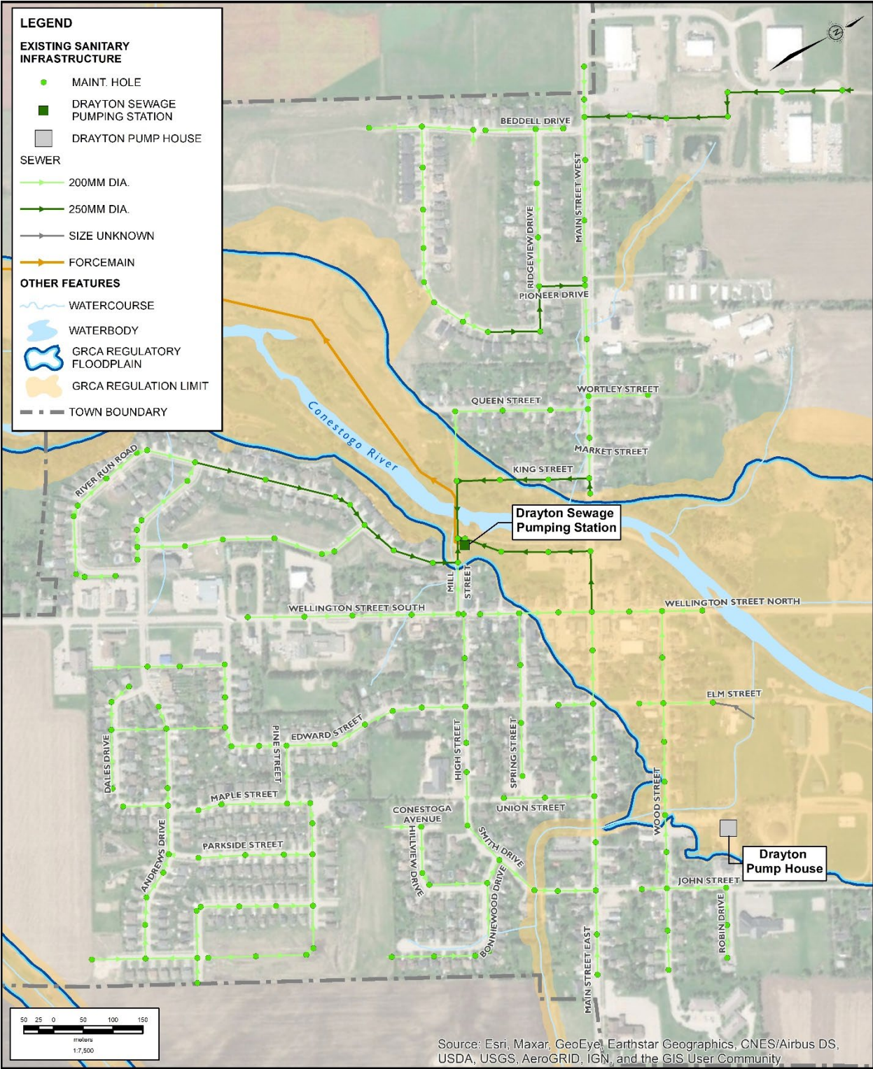
Figure 5-3: Drayton Wastewater Collection System
