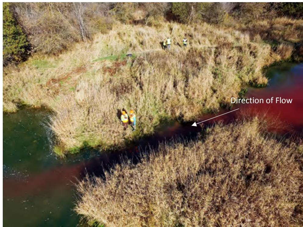
Photo B. At receiving channel discharge point to Conestoga River. Dye tracer at about 25 minutes in to the study; dye has not yet filled pond completely and has only begun entering the River.
