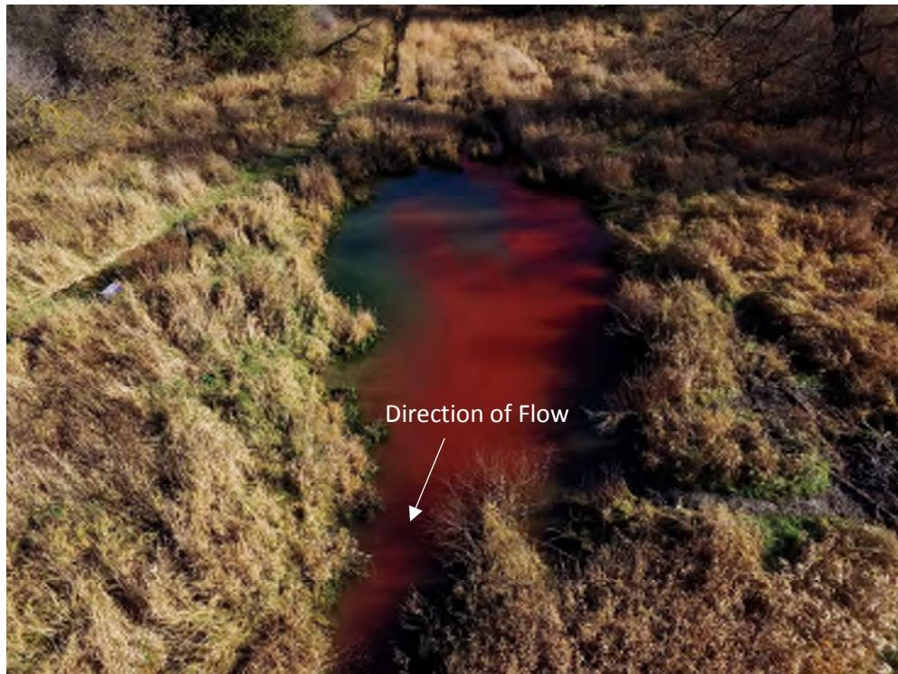
Photo A. Small pond in receiving channel just upstream of discharge point to Con estoga River. Dye tracer at about 25 minutes in to the study; dye has not yet filled pond completely.
